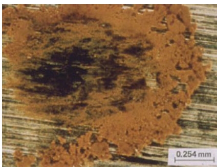
Figure 2 | Fretting corrosion of steel in air produces the red iron oxide hematite ( \text{Fe}_2\text{O}_3 ), where the wear scar is surrounded by red iron oxide.
